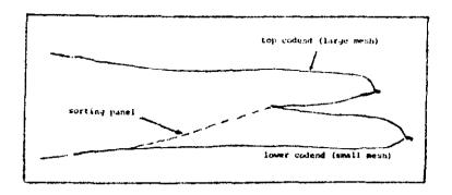
The theory of the net was that the shrimp would pass through the large mesh panel into the small mesh codend. It is known that fish will try to avoid nets; so, as the fish encounter the panel they will swim along it rather than go through it. That will funnel them into the large mesh codend. There the little fish will pass through the larger meshes as they get tired swimming or as they get crowded into it when the bag begins to fill up.
