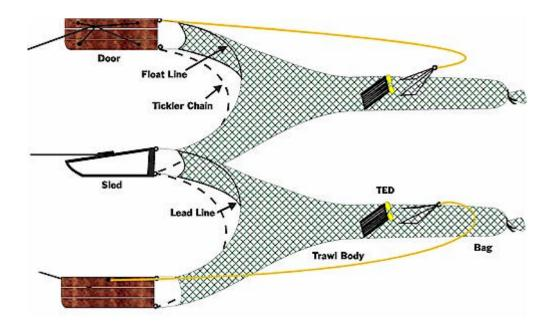
Comparative trawl tows were conducted aboard the 46-ft single diesel powered F/V Erin Lynn captained by Terry Ricks (TSPA). Tows were made with a control trawl attached to one outside door and then to the metal sled, while the BRD trawl was attached to the other door and the metal sled (Figure 4). Vessel speed was 2.5 knots. Tow time was set at 1 hour from lock-down of winch to the beginning of retrieval.
