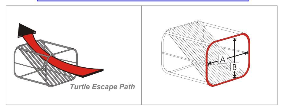
The front hoop on a inshore hooped hard TED must have an inside horizontal measurement of at least 35 inches (89 cm) **[A]** and an inside vertical measurement of at least 30 inches (76 cm) **[B]**.
