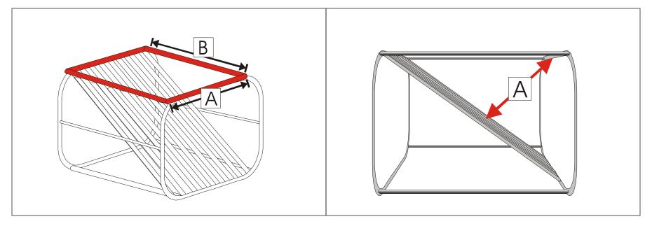
An inshore hooped hard TED the escape opening must have a horizontal measurement no less than 35 inches (89 cm) wide **[A]** and a forward measurement no less than 20 inches (51 cm) **[B]**. The clearance between the deflector bars and the top of the front hoop must be at least 20 inches (51 cm) **[A]**.
