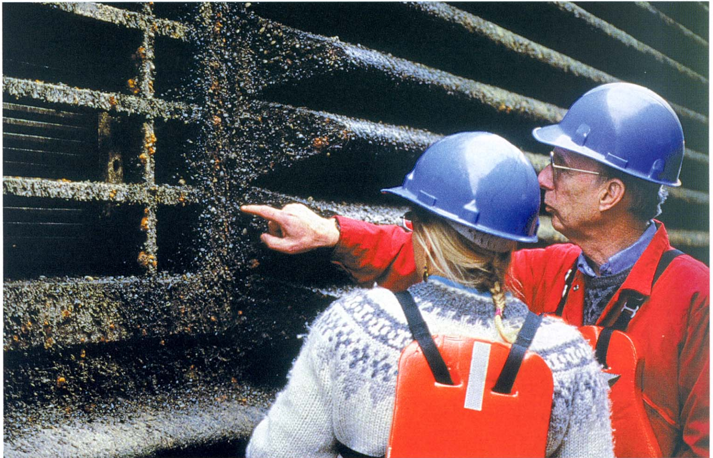
Yvonne Allen and an unidentified shipyard worker examine zebra mussels infesting recesses on a towboat's keel coolers.
